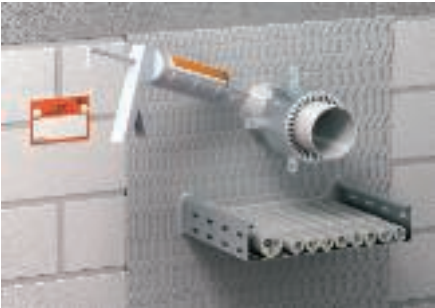
Mount the suitable pipe seal on the pipe, on both sides in the case of wall insulation, only on the underside for ceilings. The flange may not protrude beyond the edge of the insulation. Seal the pipe with fire protection filler.
