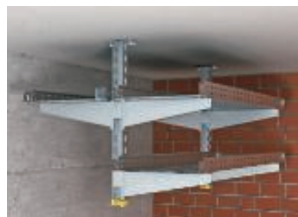
One to three-layer mounting variant, mounted on both sides, with US5K suspended support and 400 mm tray widths.
