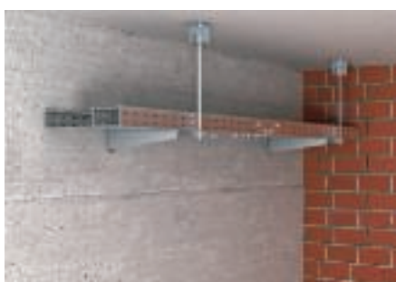
One-layer standard support construction as wall mounting with SKS cable tray and threaded rod locking vertically to the ceiling.
