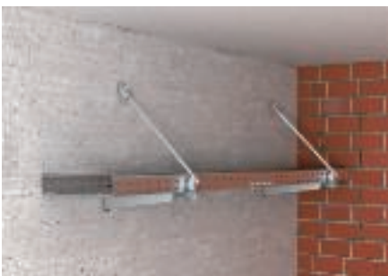
One-layer standard support construction as wall mounting with SKS cable tray and threaded rod locking diagonally to the wall.
