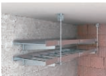
Two-layer cable-specific support construction for wall mounting with SL60VS/F cable ladders, with threaded rod locking vertically to the ceiling.
