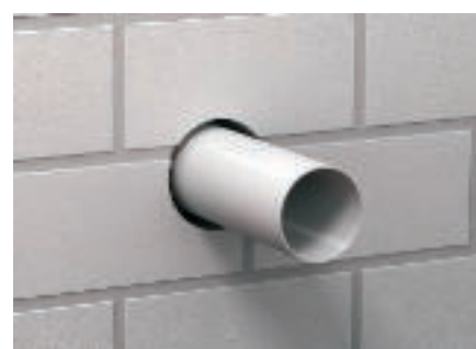
The pipe seal can be used with wastewater pipes made of various plastics (for details, see the approval). If there is a fire, it ensures safe, smoke-gas-proof closure of the opening.
