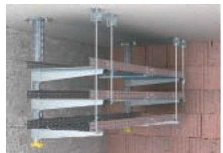
Three-layer cable-specific support construction made of EKS cable trays with U suspended support, bracket mounted on one side. The third layer (lower cable tray) must be locked with a separate threaded rod.
