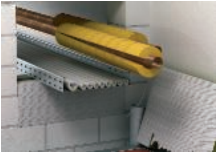
Continuous path insulation mounting on the non-combustible pipes. Refer to the approval for the length, thickness and material. The path insulation of the individual pipes may touch.
