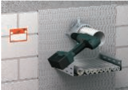
Drill through the two mineral fibre plates (for M6 or M8 threaded rods). Use the flange of the pipe seal as the drilling template.
