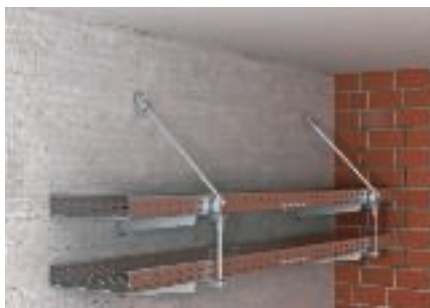
Two-layer standard support construction as wall mounting with SKS cable trays and threaded rod locking diagonally to the wall.
