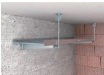
One-layer cable-specific support construction for wall mounting with SL60VS/F cable ladders, with threaded rod locking vertically to the ceiling.
