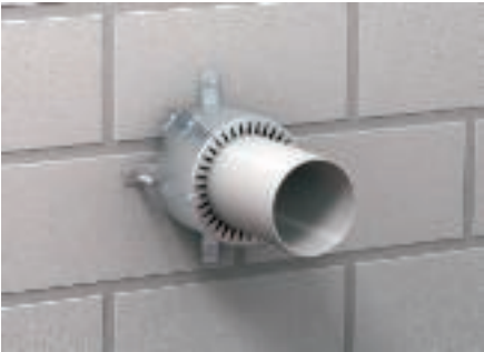
In solid walls, mounting takes place with approved metal anchors. Threaded rods are mounted using the push-through method in lightweight partitions. The bent holding straps can be used as a drilling template.
