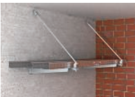
One-layer standard support construction as wall mounting with SKS cable trays and threaded rod locking diagonally to the wall.
