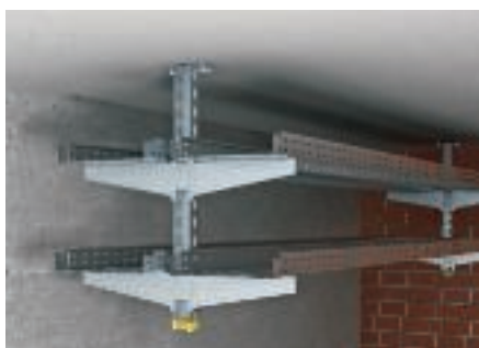
One to four-layer mounting variant with US5K suspended support and tray widths to 300 mm.
